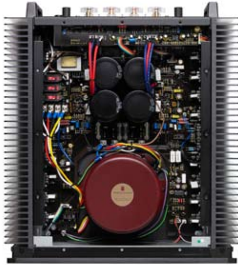
Parasound Halo A-21+ Power Amp $3195 New AUDIO POWER increased from 250 to 300w 8 ohms AUDIO POWER increased from 400 to 500w 4 ohms AUDIO POWER increased from 750 to 1000w bridge 60 amperes of current; staple with 2 ohm loads Balanced inputs; JFET input and MOSFET drivers 16 beta matched 60 MHz 15 amp bipolar outputs Multiple power supplies, full power down to 5Hz
